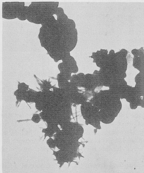
Figure 9. Amorphous type insoluble gum from desert aged jet fuel
